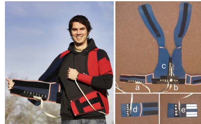
figure 1. Tactile vest and arm straps. Left picture © Bram Saeys. Letters indicate the actuators for the stomach (a), lower (b) and upper back (c), upper arm (d) and wrist (e).
